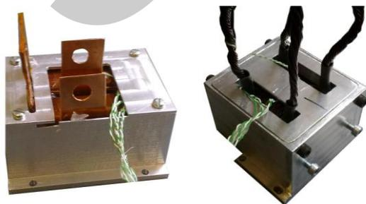
Figure 10. Magnetic components in aluminium heat-sinks
