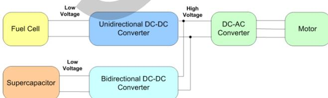
Figure 1. Traction System Architecture
