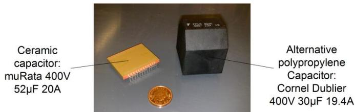
Figure 8. Capacitor comparison
