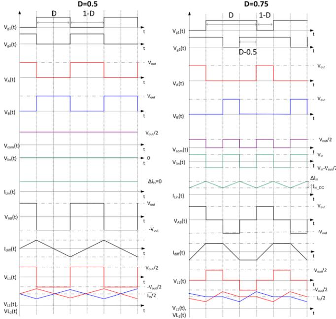
Figure 3. Dual interleaved boost with IPT waveforms
