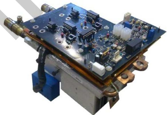
Figure 12. Converter prototype
