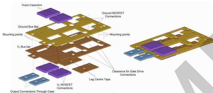
Figure 9. Bus-bar and capacitor module
